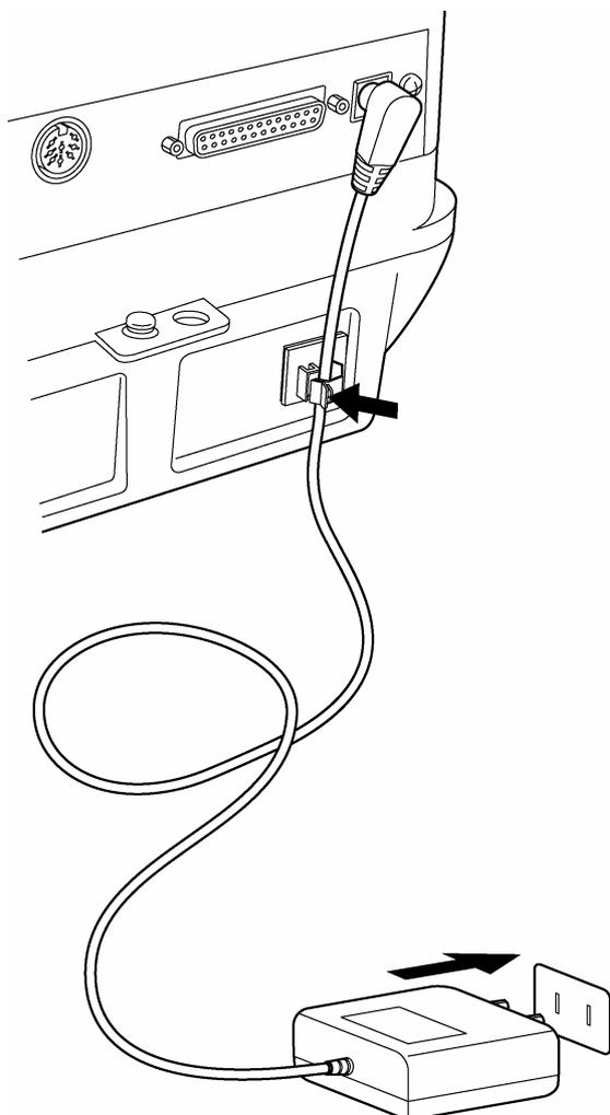
1. Supply power to balance via mains adapter. After the balance performs a self check, calibration will be automatically executed. During this process, the display will change as follows. "CHE 5", "CHE 4" ..... "CHE 0", "CHE 2", "CHE 1", "CAL 2 – CAL 0", "CAL-End", "oFF". This adjustment can be interrupted immediately after switching-on the power supply by actuating the **[ON/OFF]**-key. However, at least one adjustment must be carried out before the balance can be used.
