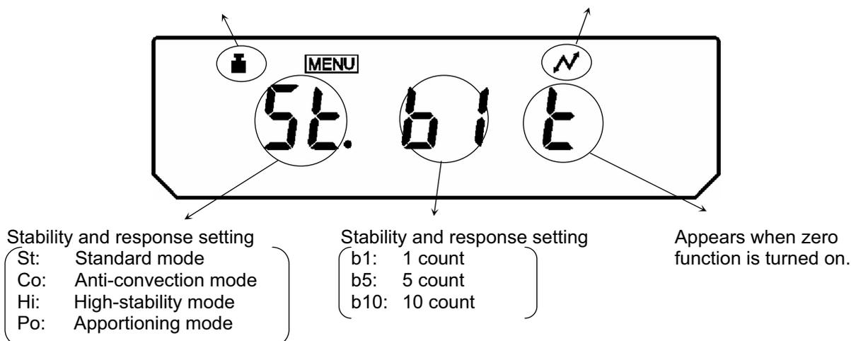
The weight symbol is displayed when either automatic adjustment PSC or Clock-CAL or both functions are turned on.
