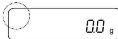
If the display shows the stability display **[o]** the balance is in a stable status. The **[o]** indication disappears if the condition is unstable.
