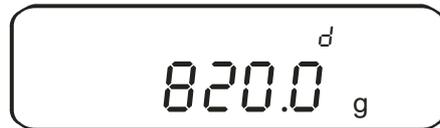
**2. Sample weight in the measuring liquid**
