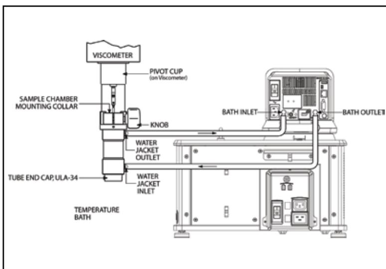
4. The water jacket is connected to a circulating water bath as shown in Figure 6. For temperatures from  $-15^{\circ}\text{C}$  to  $65^{\circ}\text{C}$ , gum rubber tubing (Brookfield Part No. EX-TUBING) is used. For temperatures from  $65^{\circ}\text{C}$  to  $100^{\circ}\text{C}$ , Fluran<sup>®</sup> tubing (Brookfield Part No. ULA-45) should be used.
