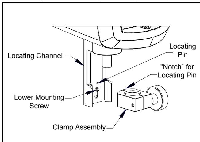
2. Attach the clamp assembly to the locating channel, as shown in Figure 4, by screwing the lower mounting screw on the locating channel into the hole at the back of the clamp assembly.
