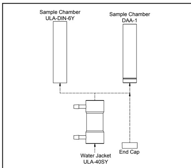
**Figure 6: Installing the Water Bath**
