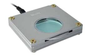
The BL-ZW1 is a backlight accessory which opens up a whole new range of applications. The backlight has a built-in, freely rotatable polarizer that works in combination with the Dino-Lite polarizing microscopes such as AM4113ZT, AM4013MZTL or AM7013MZT. The BL-ZW1 offers a light intensity over 5000 mcd.
