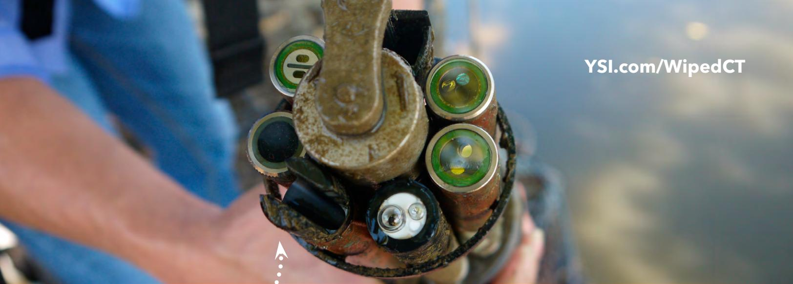
Most conductivity cells cannot be fully cleaned by mechanical anti-fouling wipers, but the **EXO Wiped (C/T) Smart Sensor** was purpose-built to protect your conductivity data.
