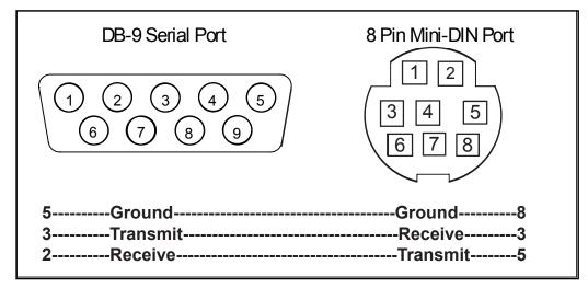
Mini-DIN to DB-9 Connection for RS-232 Signals
