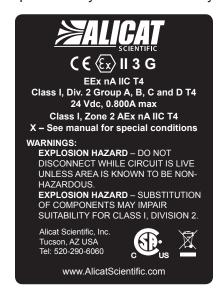
USE of Alicat instruments (M, MC, MS, MCS, MCR, P, PC and PCR product families only) in applications requiring ATEX Certification.
