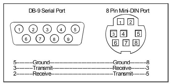
Figure 2. Mini-DIN to DB-9 Connection for RS-232 Signals
