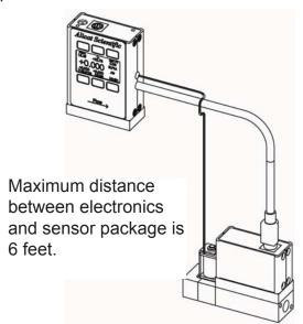
In these applications we recommend our custom gauge calibration at a gas temperature of up to 70°Celsius. This will reduce zero shift errors that occur when actual gas flow temperatures deviate substantially from the gas calibration temperature. This configuration is also used in integrations that require a compact flow package at the installation point.
