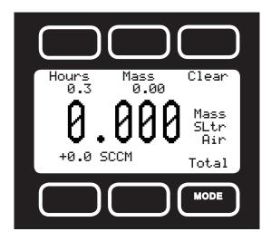
**Counter** – The counter can have as many as six digits. At the time of order, the customer must specify the resolution of the count. This directly affects the maximum count. For instance, if a resolution of 1/100ths of a liter is specified on a meter which is totalizing in liters, the maximum count would be 9999.99 liters. If the same unit were specified with a 1 liter resolution, the maximum count would be 999999 liters.
