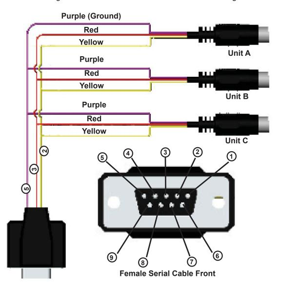
Figure 3. Typical Multiple Device (Addressable) Wiring Configuration
