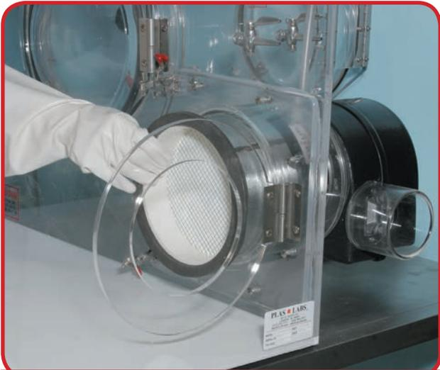
800-HEPA/S with filter access door open. Internal view (when changing filters)
