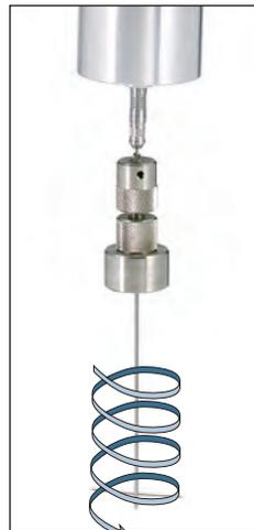
For viscosity/consistency measurement of gels, pastes, creams, putty, gelatin and other non-flowing substances.
