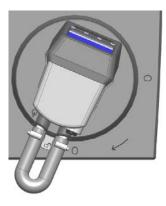
3. Lift the Controller straight up and out of the opening of the Circulator's top deck.
