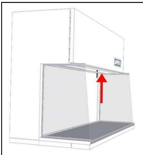
Figure 12 Position of the FL-tube
