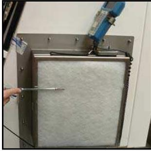
Figure 23 Measuring the inlet velocity of the MSC III
