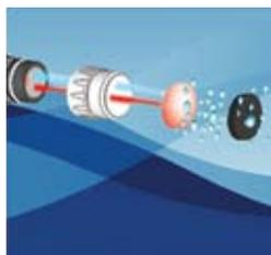
With ODO technology, oxygen is constantly moving through the diffusion layer, affecting the luminescence of the sensing layer.
