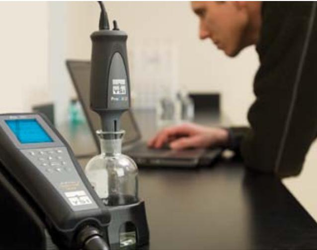
The ProODO utilizes “smart” sensor technology which stores calibration data within the sensor. This allows probes to be placed on any ProODO instrument without re-calibration.
