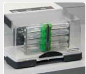
Grinding jars of polystyrene are also available for the mixing of solid sample materials.
