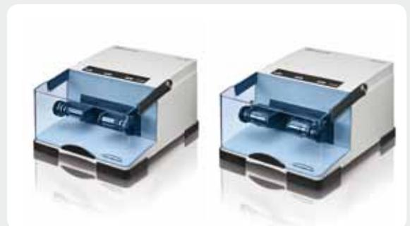
**RETSCH Mixer Mills** are used for the pulverization of **hard, medium-hard, soft, brittle, elastic and fibrous materials**. The sample feed size depends on the mill and can be as large as 8 mm. If the feed size is larger than this then the sample must first undergo preliminary size reduction.
