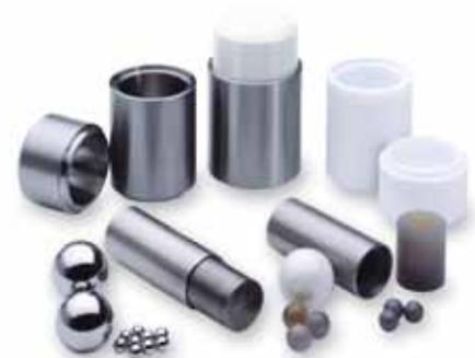
Grinding jars with push-fit lids for MM 200
