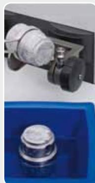
The CryoKit is a cost efficient solution for occasional cryogenic grinding with the Mixer Mill MM 400. This set of insulated containers, tongs and safety glasses is used for pre-cooling the grinding jar in liquid nitrogen.
