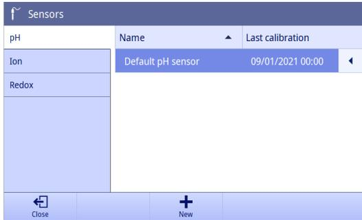
Sensors for pH, redox and ion can be connected to the instrument. One default sensor per sensor type is predefined. Each method can only select the sensors with the matched sensor type.
